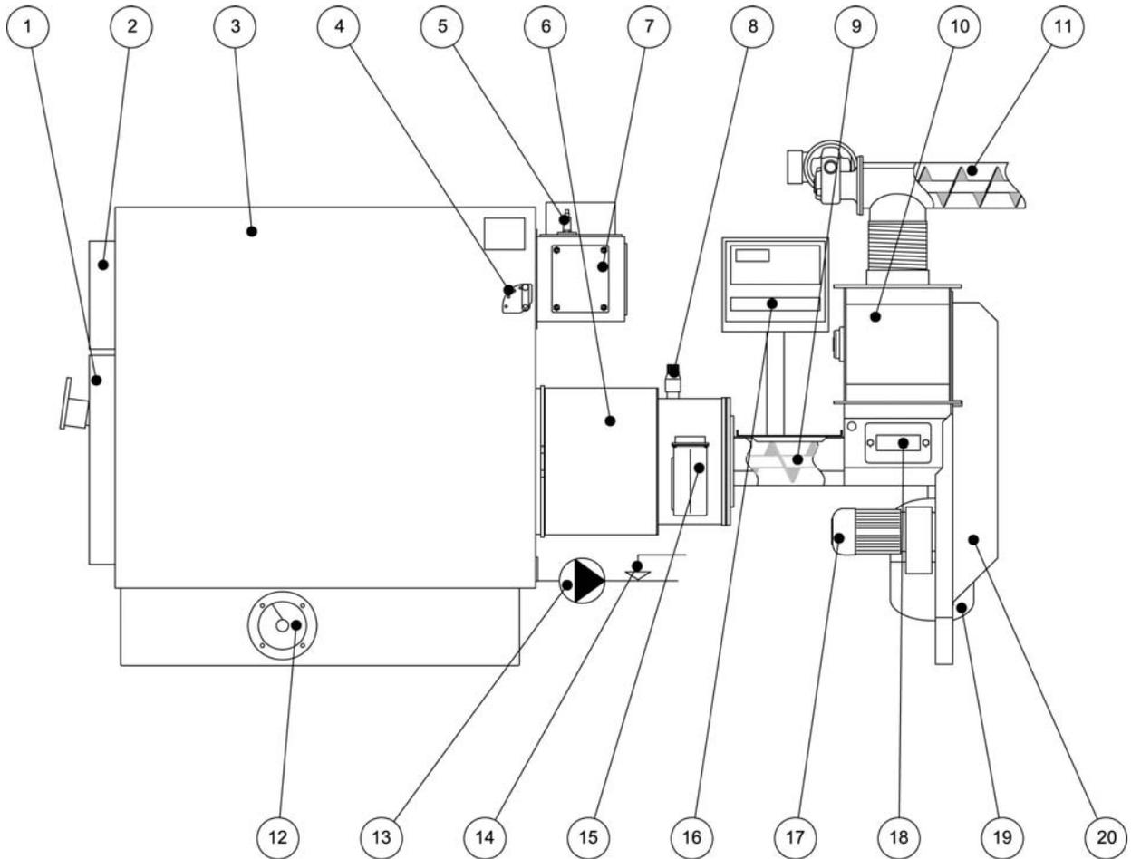
1. Boiler door with inspection glass/draft flaps, depending on model
