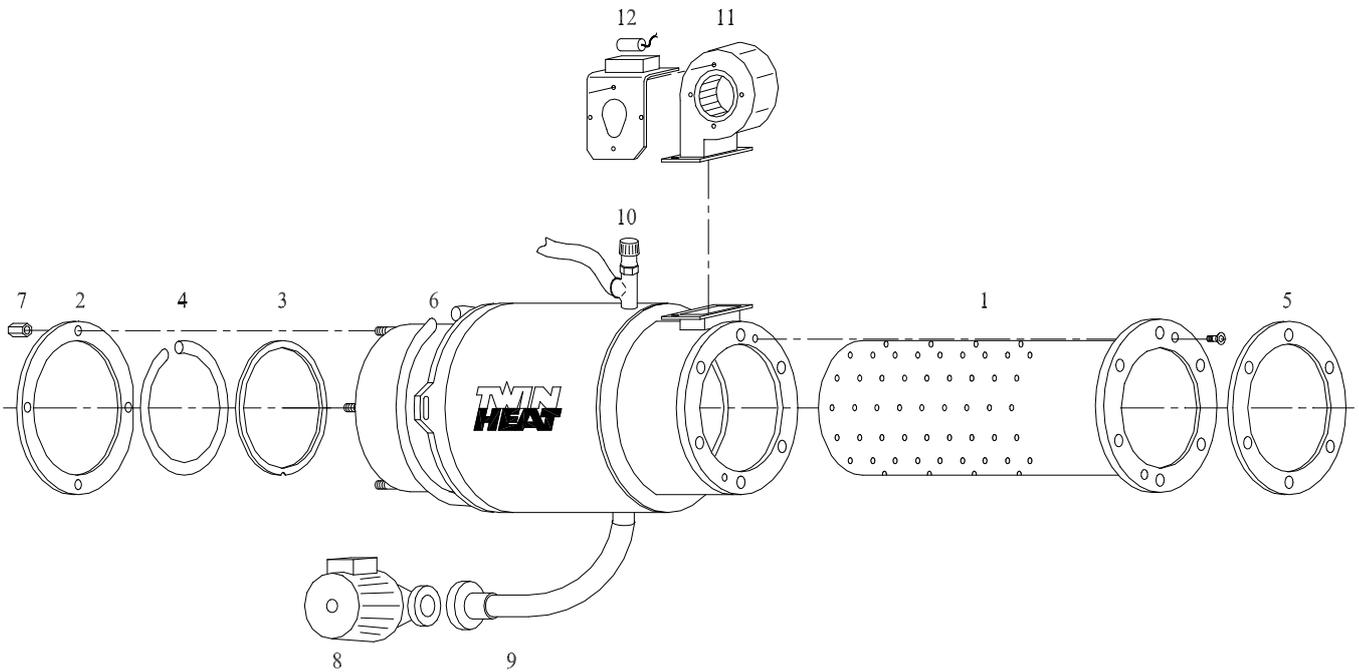
**8.2 Parts list burner tube M40**
