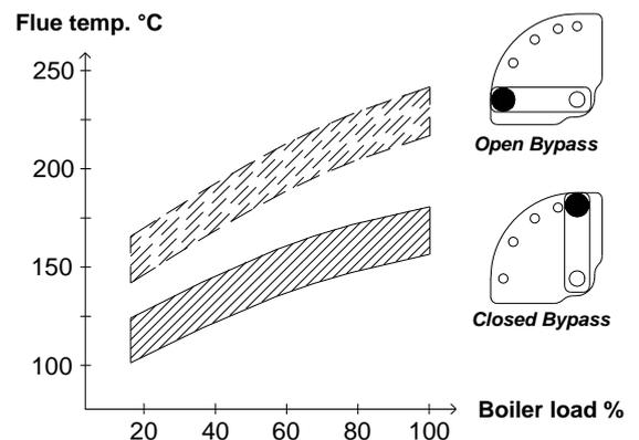
Fig. 3- Approx. flue temperature compared to boiler load
