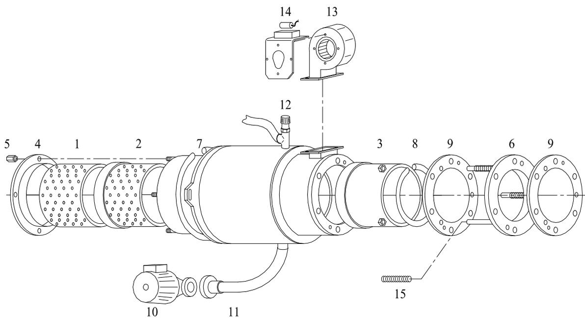
**8.3 Parts list burner tube M80**
