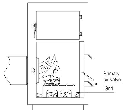
Fig. 6- Combined heating
