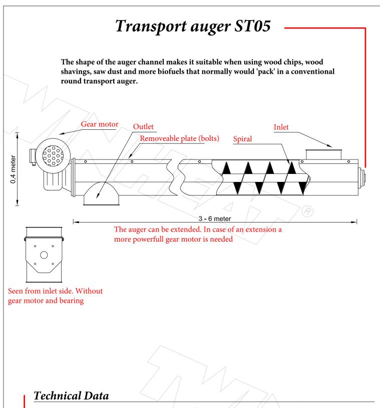
Mains connection Inlet / Outlet Capacity Suitable fuel types Gear motor 3 x 400V+0+PE, 10A OK180 / Ø180mm Depends on the fuel type Wood chips, wood shavings, sawdust and more Nordgear: 1,1 kW. 29 o/min
