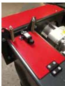
Spring loaded lid with an electrical switch, which stops the delivery auger in case of fuel piling up
