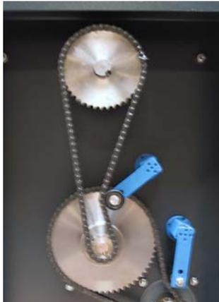
4) The chain must run as shown in this picture. Check after having finished the work, that the chain runs freely.
