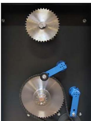
*The chain tightener should not be loosened, as it wrings in the rubber fixation*
