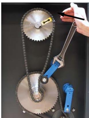
1) Place the wrench, a big thong or the like at “arm of the chain tightener and press against the cog-wheel as shown.
