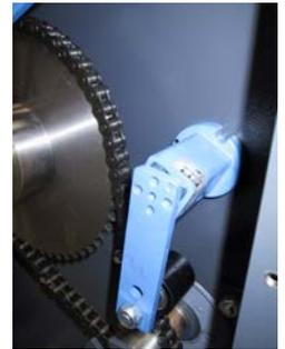
*Chain tightening device*
