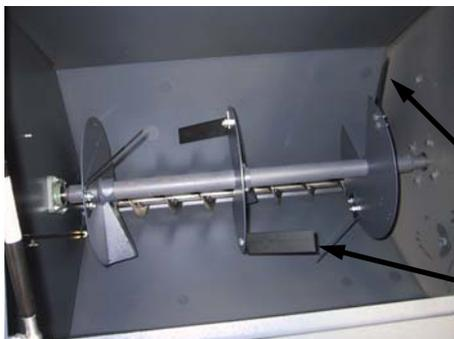
The stirrer wings included ( both long and short versions) are mounted as shown on picture. The long model must be fit on the rear side of stirrer plate – towards the chain
