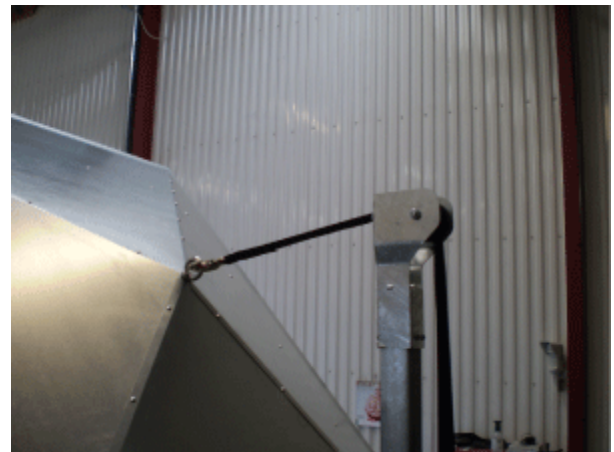
Top of the pillar with hook fixed in the eye bolt.
