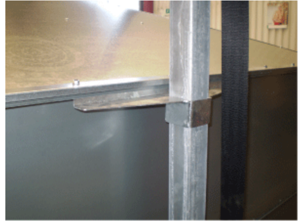
Top bracket mounted together with bolts for lower part of hinge
