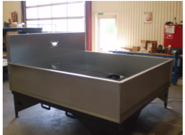
Silo base with the first section and one plate of the second section mounted
