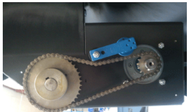
Chain connection with chain wheels, flange-bearing and chain tightener
