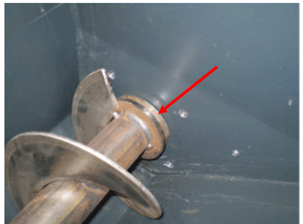
Bronze bearing on auger shaft
