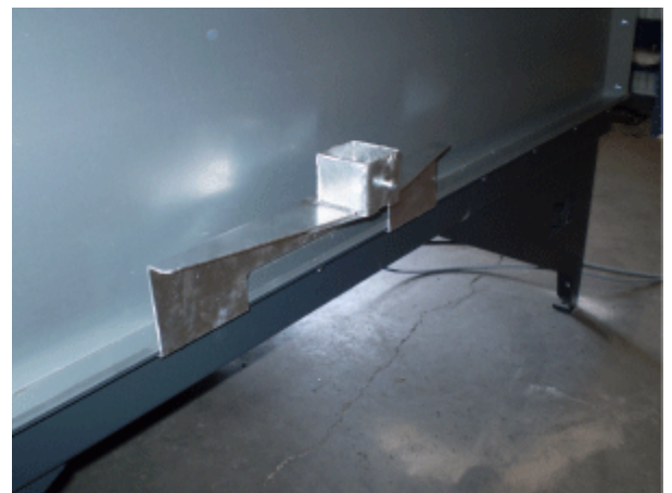
Lower bracket mounted in the centre of the silo side
